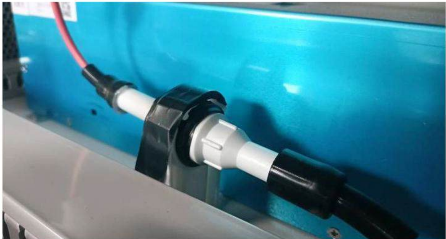
Insulation Support Frame
