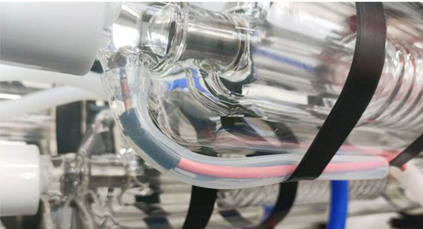
High-Voltage Wire Insulation
